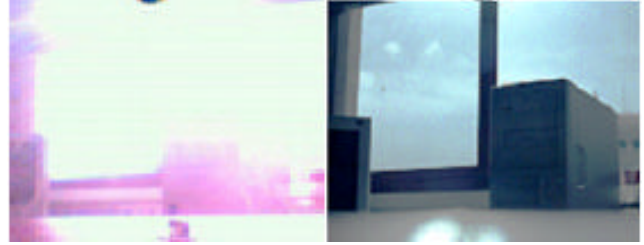
Fig. 4. A view of a window in a shiny day. CCD camera (left) gets saturated, losing details that can be observed with a logarithmic camera (right).
